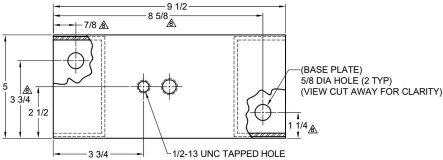
**TYPE MH-3C SPRING ISOLATORS WITH INTERNAL ADJUSTMENT**
